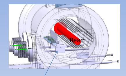
Displacement System Blade shall be mounted on linear guides to allow for same precision in positioning as on the SMH16. Motor location to be decided.
