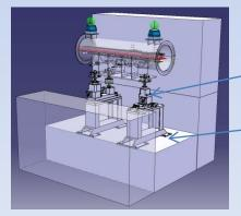
Lower supports can be dimensioned to allow installation of a shielding block under the supports, to which the lower supports could be secured.
