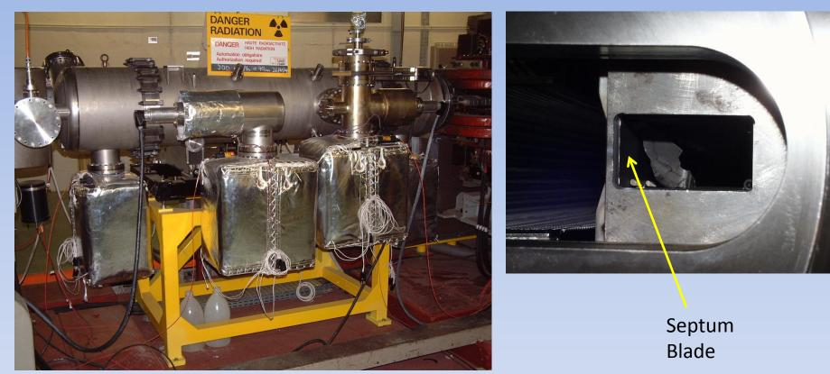
.....Since the region of the septum SMH16 has to be accessible for maintenance and repair, the present situation is far from optimal. A proposal has recently been made during the MTE workshop to strongly reduce the radiation level in this region. The idea is to install a dummy septum blade inside the straight section 15, to shadow the coil in the 'real' septum inside the straight section 16.
