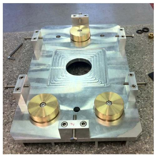
Limit switch actuators and adjustable feet for vacuum vessel Feet allow for x,y,z adjustment and permit plug n play principal for the vacuum vessel.
