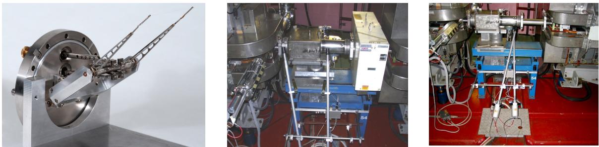
Fig. 26: Schematic layout of the mechanism of the PS wire scanner (left). The installation of the scintillators on one side of the vacuum chamber used during the experimental campaign and the new layout with symmetric scintillators are shown on the centre and right part, respectively.
