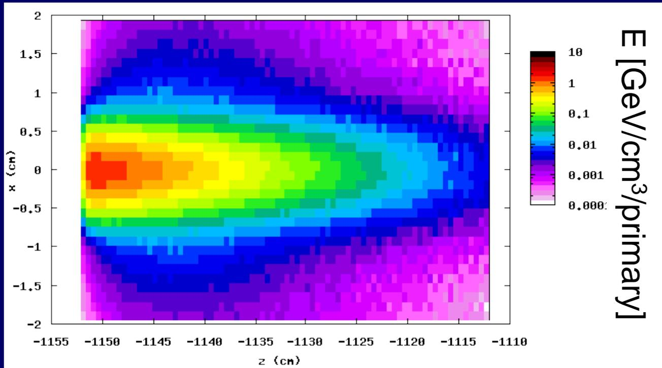
projection of deposited energy  $E$  [GeV/cm<sup>3</sup>/primary] into the x-z plane, averaged over the blade thickness  $\Delta y=3\text{mm}$
