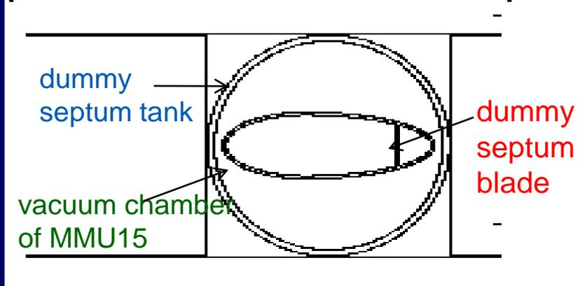
**dummy septum blade** : 40 cm length, 3mm thickness and 3.88 cm height ; material: tungsten
