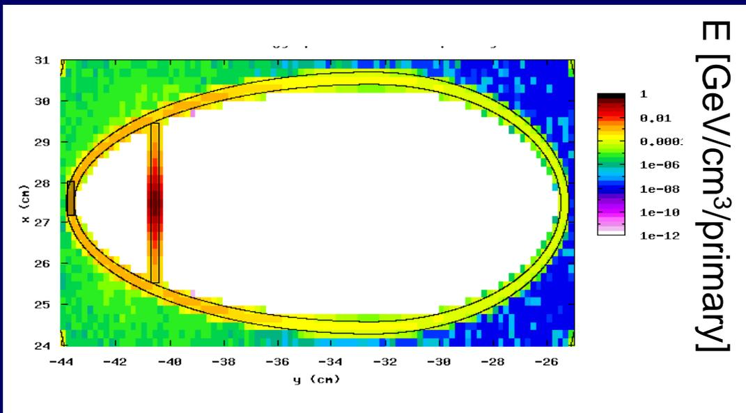
2-dimensional projection of  $E$  [GeV/cm<sup>3</sup>/primary] in the x-y plane, averaged over  $-1144 < z < -1122$  cm
