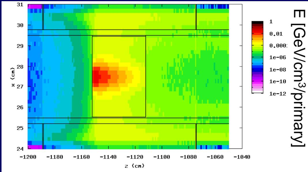
2-dimensional projection of  $E$  [GeV/cm<sup>3</sup>/primary] in the x-z plane, averaged over  $-44 < y < -24$  cm (z range here length of SS15)
