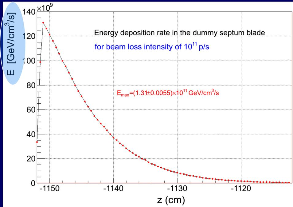
1-dim projection along the blade length ( $z$ ),
