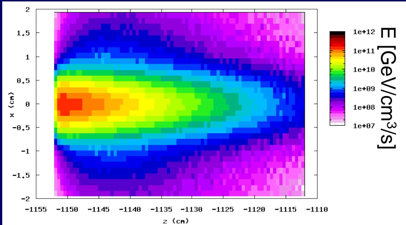
projection of deposited energy rate  $E$  [GeV/cm<sup>3</sup>/s] into the  $x$ - $z$  plane, averaged over the blade thickness  $\Delta y=3$ mm
