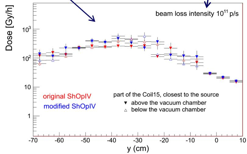
addition of 10 cm shielding further upstream, in between the vacuum chamber and the coils of MMU14, reduces the dose inside the coils14 by a factor of 2.5
