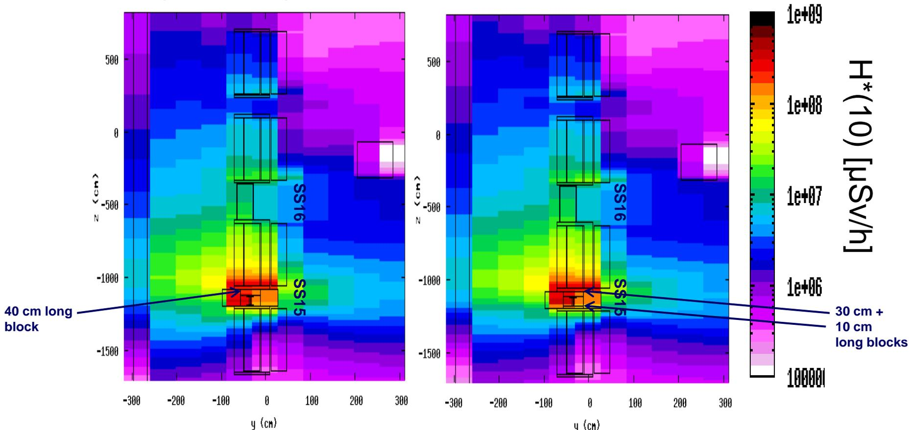
Ambient Dose-eq Rate [ $\mu\text{Sv/h}$ ] in z-y plane averaged over 2 m height (x)
