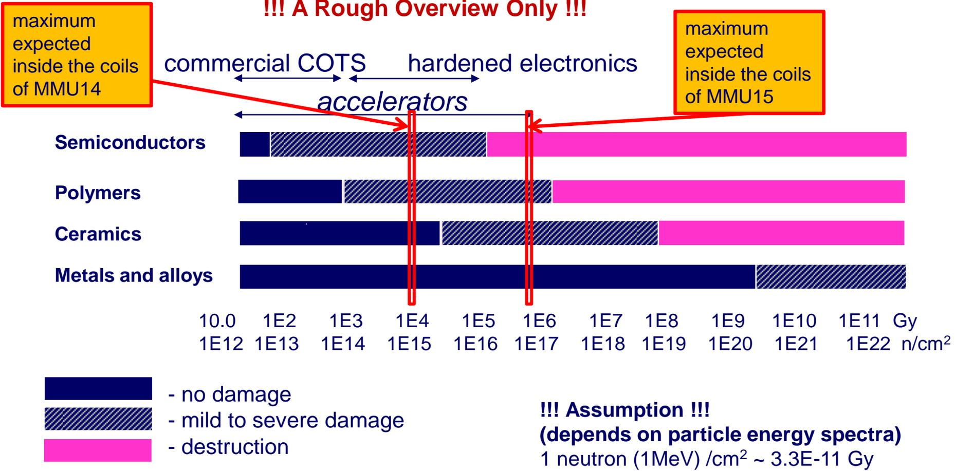
Since the maximum radiation level expected inside the coils of MMU15 is very high, there is not much sense in reducing the downstream part of the shielding
