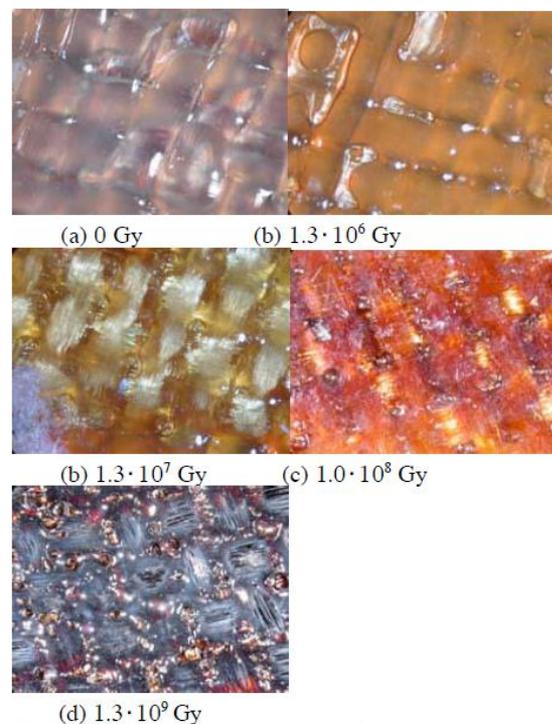
Figure 4: Test piece photographs magnified by a microscope.
