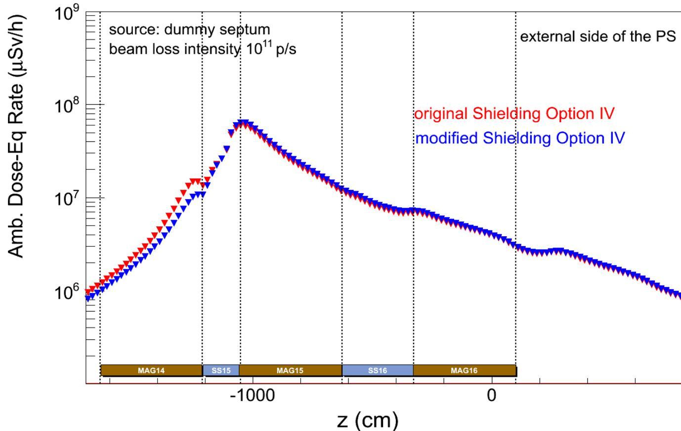
1-dim Projections of Ambient Dose-eq Rate [ $\mu\text{Sv/h}$ ] along z
