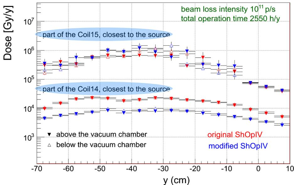
Radiation dose in the coils of MMU15 higher by factors of 25-60 compared to coils of MMU14
