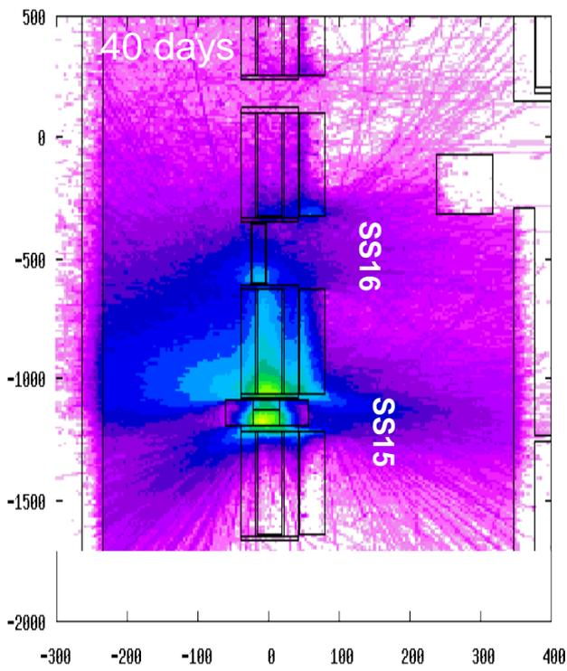
2dim projections of  $H^*(10)$  in y-z plane at the beam level
