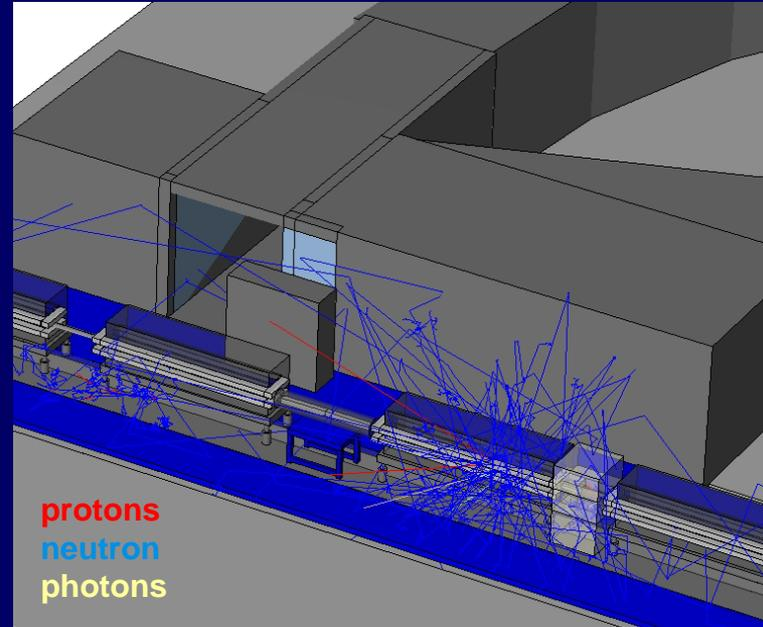
Secondaries produced lead to an elevated dose in the tunnel
