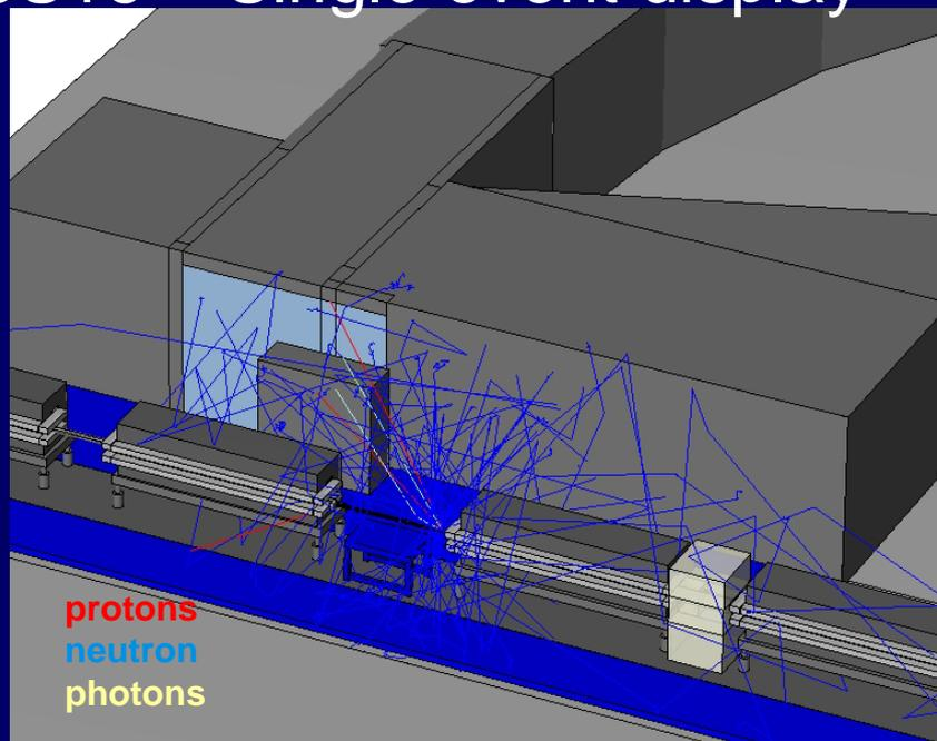
Secondaries produced lead to an elevated dose in the tunnel
