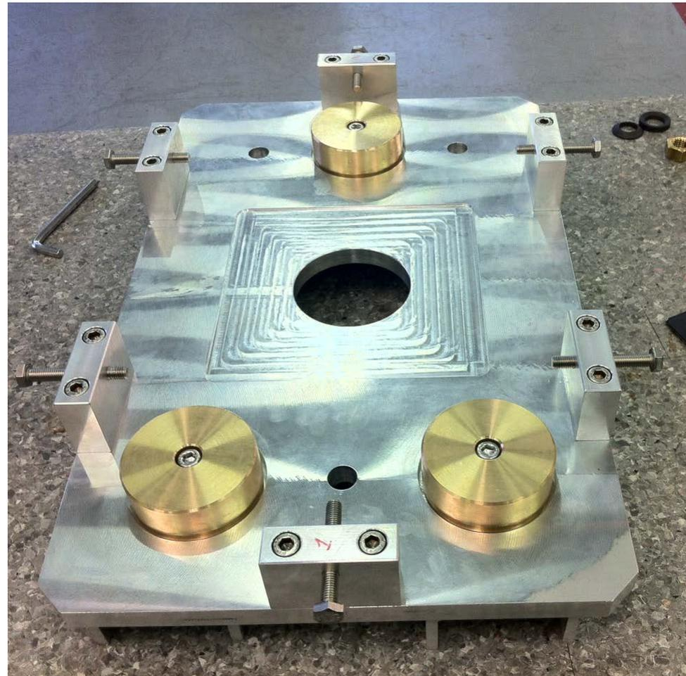
Limit switch actuators and adjustable feet for vacuum vessel
