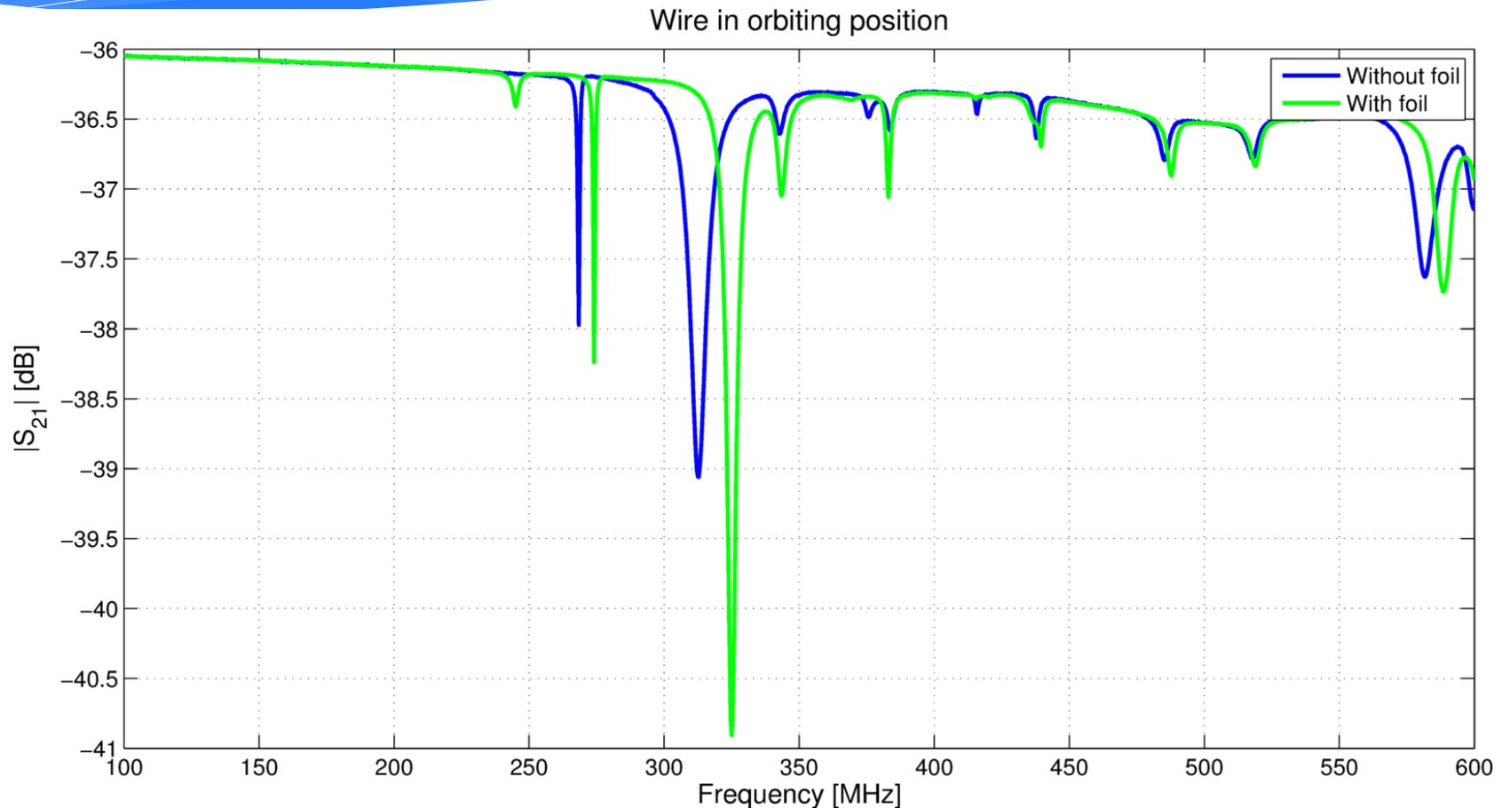
To verify the correct behaviour of the fingers, we tried to obtain insulation between the screen and the support with a foil. Using the insulation a lower frequency peak (230 MHz) is generated.
