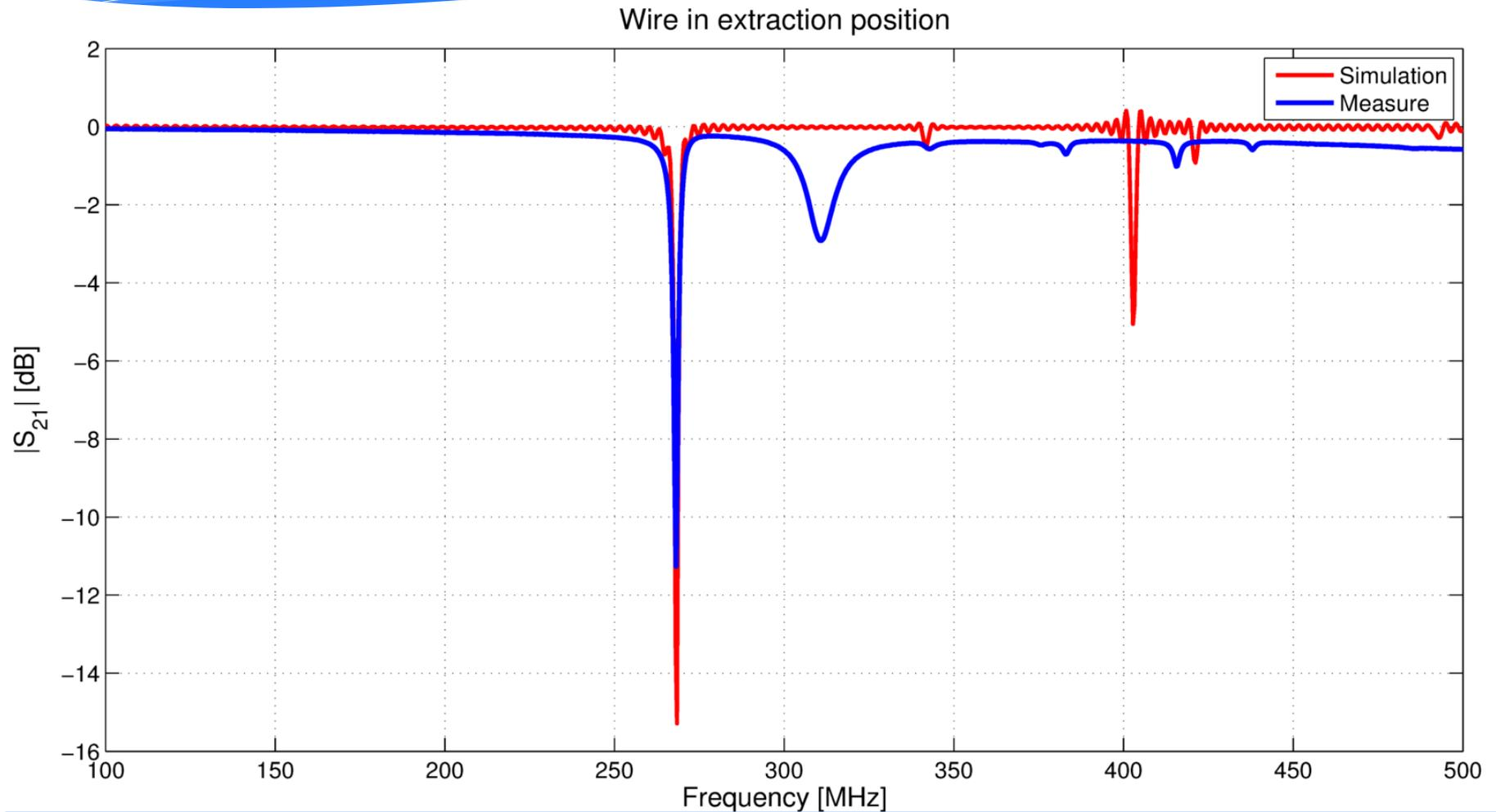
Measurements have been compared with simulations in time/frequency domain. Both measurement and simulation agree on the first trapped mode at the frequency of 270 MHz. The fingers are working well on low frequency mode cancelling.
