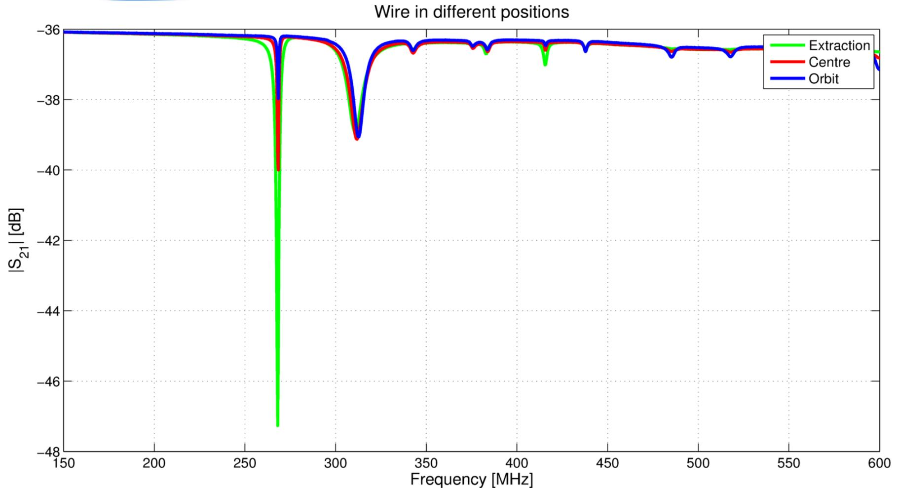
The 270 MHz mode is generated by resonances due to the space (3mm) between screen and blade. Measurements confirm what observed in simulations, that during extraction increases the amplitude of this mode.
