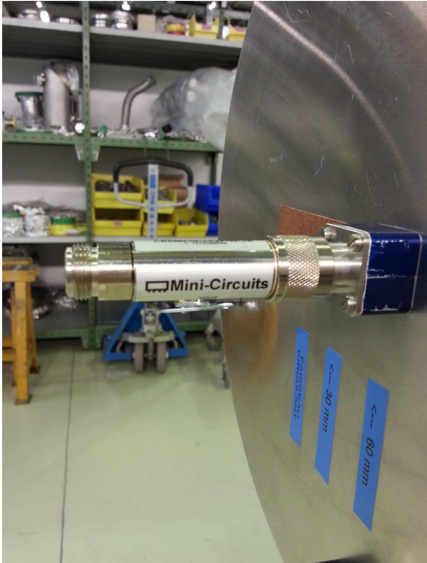
x2 10 dB attenuators have been used for both measurements
